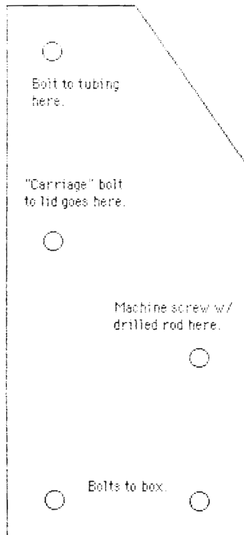
Figure 3. Pattern for plywood (Scale: 1 1/2" = 1') used for seatback and drawing of brass rod with hole drilled to use on Econoline third seat.
